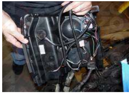
Step 22: Connect the wire harness to the new Anzo headlight and reverse steps to put headlight back in place.
