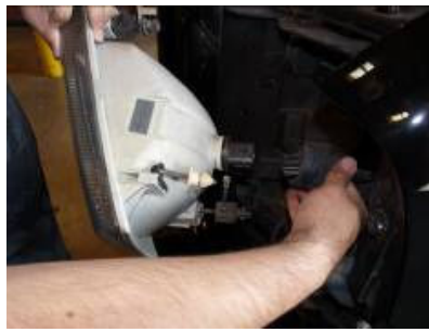
Step 11: Unclip the head light wire harness.
