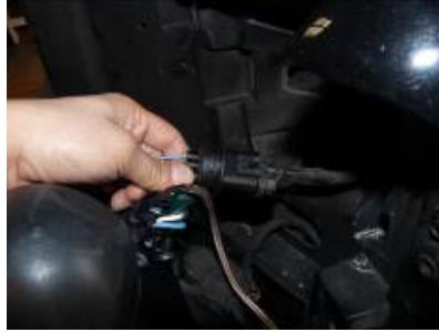
Step 14: Plug in the head light wire harness into the new Anzo light.
