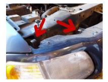
Step 2: Pull up the two locking pins holding in the headlight.
