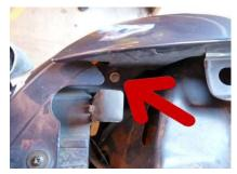
Step 4: Use the t20 torque screw to remove the screw holding in the corner light.
