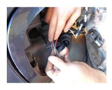
Step 8: Splice the led wires into the corner light. Blue wire (+) will be positive splice into the brown wire on the corner light. Black wire (-) negative will be spliced in to the black wire on the corner light.
