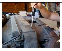
Step 1: Remove the eight plastic screws holding in the plastic cover shroud.
