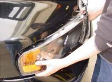
Step 10: Slide the new ANZO headlight into the housing.
