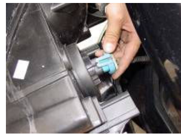
Step 9: Plug the headlight socket to the bulb.
