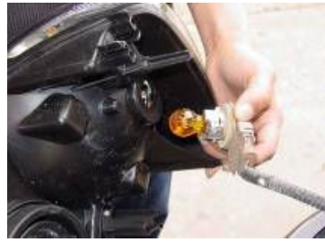
Step 8: Place the turn signal bulb into the new Anzo housing.
