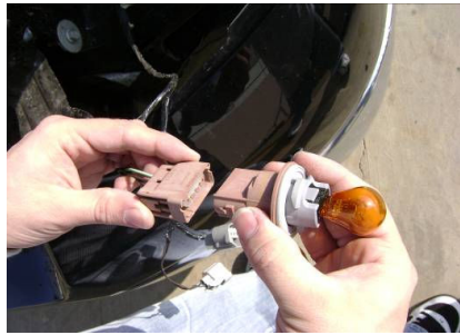
Step 10: Disconnect the inner signal bulb socket from the wire harness.
