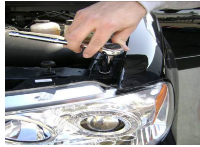
Step 20: Tighten up the three 10 mm bolts that hold the headlight to the housing.
