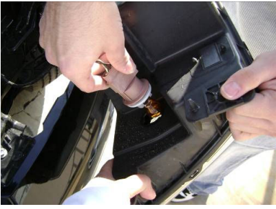
Step 6: Twist and pull the inner turn signal bulb out of the housing
