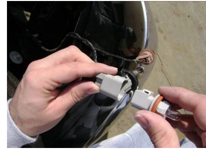
Step 11: Disconnect the side marker socket from the wire harness.
