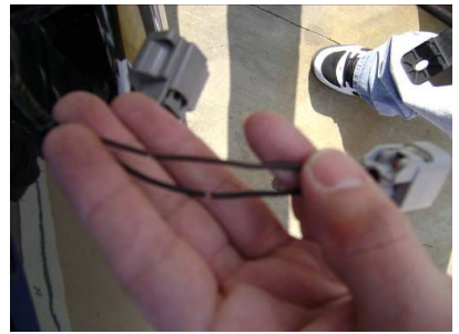
Step 13: locate the side maker light, pull back the electric tape exposing the black and brown wire on the stock harness.
