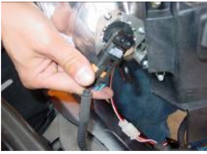
Step 7: Plug the headlight harness to the ANZO headlight
