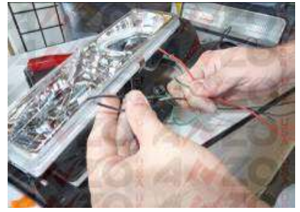
Step 13: Connect the red and blue wire together and the black with black.
