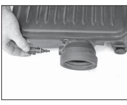
20. Twist the air temperature sensor counter clockwise and remove it from the stock intake plenum.
