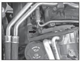
14. Remove the rear, lower A/C compressor mounting bolt shown.
