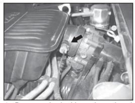
4. Depress the locking tab on the air temperature sensor electrical connection and disconnect the electrical connection.
