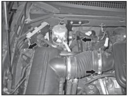
2. Loosen the hose clamp at the intake plenum and the air box mounting nut. Then disconnect the crank case vent from the inline fitting.
