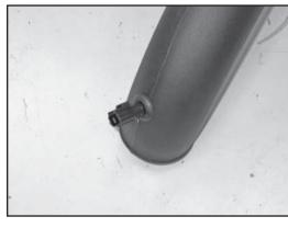
22. Install the air temperature sensor into the grommet installed into the K&N Intake Tube in step #19.
