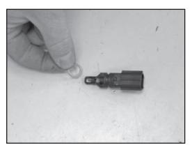
21. Remove the "O" ring from the air temperature sensor.
