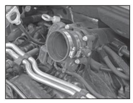
17. Install the provided silicone hose (084036) onto the throttle body and secure with the provided hose clamps.
