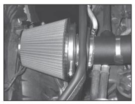
28. Install the air filter assembly onto the K&N Intake Tube and secure with the provided hose clamp.
