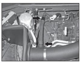
25. Install the provided silicone hose onto the 1/4npt fitting installed in the K&N Intake Tube and then attach the open end onto the hose to the factory crank case tube.
