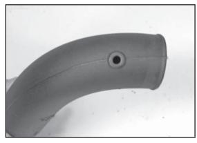
19. Install the provided grommet into the K&N Intake Tube as shown.
