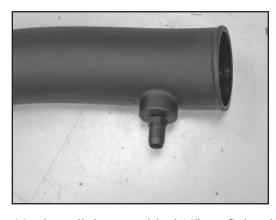
18. Install the provided ¼"npt fitting into the K&N Intake Tube as shown.
