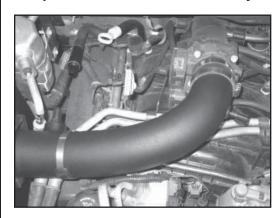
23. Install the K&N Intake Tube into the into the silicone hose on the throttle body and position so the tube aligns with the saddle clamp. Secure the tube with the provided hose clamps.
