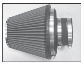
27. Install the silicone hose (08698) onto the air filter adapter as shown and secure with the provided hose clamp.
