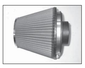
26. Install the provided filter adapter into the K&N Air Filter and secure with the provided hose clamp.
