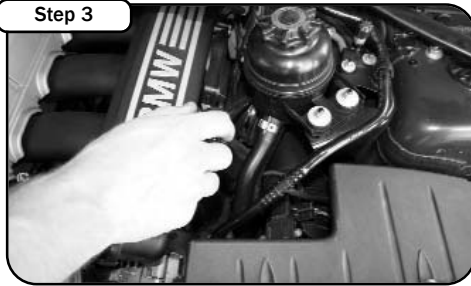
Step 3 Loosen the hose clamp on the air box, and loosen the hose clamp on the intake manifold.
