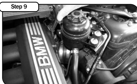
Step 9 Slide intake tube onto the manifold, and secure clamps
