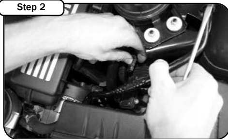
Step 2 Disconnect the MAF sensor.
