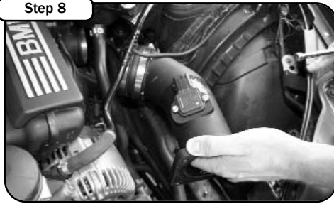
Step 8 Insert the MAF sensor assembly into the intake duct. Use the supplied gasket and screws. Secure the coupler to the intake tube using the #56 hose clamps. Do not tighten.
