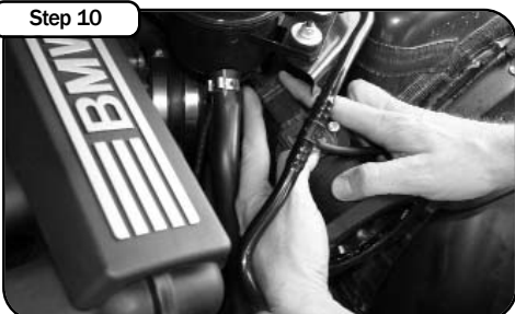
Step 10 Re-connect the MAF sensor plug.
