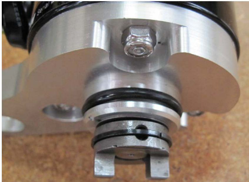
Figure 4. EPM with Shim, Drive Gear, Pin, and Retaining Clip Installed
