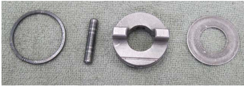
Figure 3. Retaining Clip, Pin, Drive Gear, and Shim (left to right) Removed from Distributor
