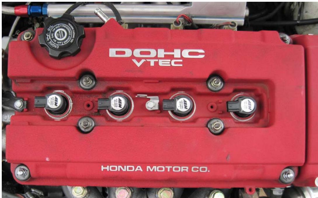
Figure 6. Coils Installed in Cylinder Head
