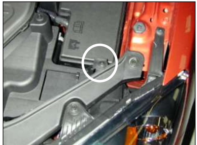
b. Remove the plastic screw connector holding the battery cooling duct in place. Remove the battery box cover and remove the battery cooling duct.
