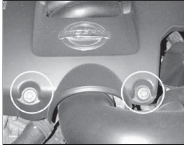
b. Remove the two screws securing the engine cover and remove the cover.
