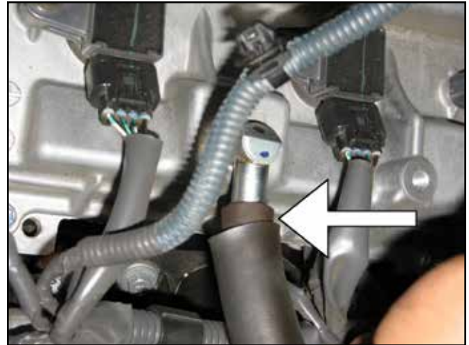
l. Disconnect the opposite end of the 5/8" ID hose disconnected in step 2f.
