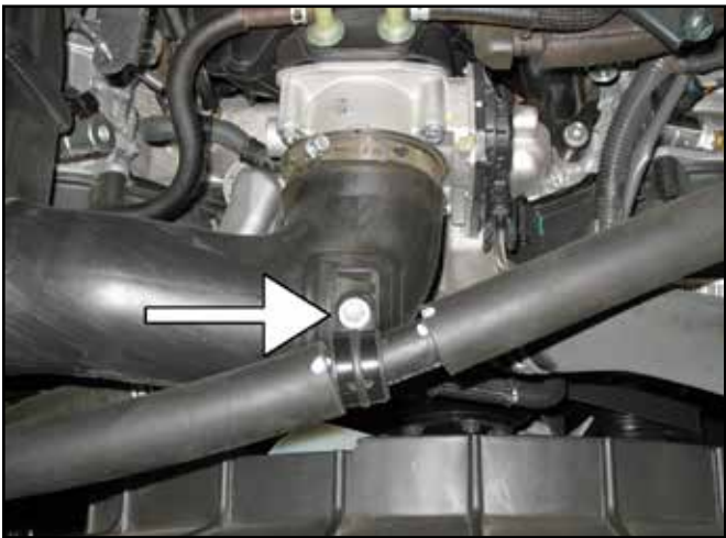
c. Remove the bolt that secures the line secured to the stock intake tube. Keep this bolt for later use.
