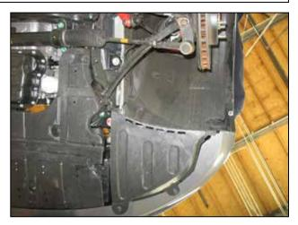
q. Reinstall the fender liner and wheel.
