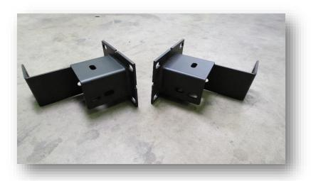
3. Passenger side has radius index, and driver side has triangular index.
