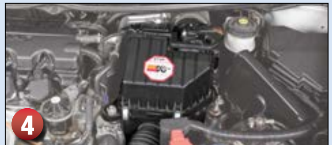
Step 4: Close the air box and apply the "Do Not Discard" decal.
