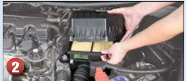
Step 2: Remove the disposable filter.
