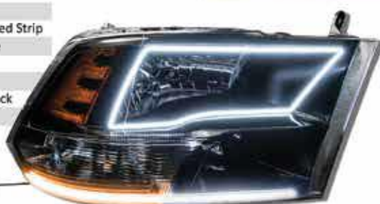
Plasma Switchback DRL installed in a Dodge Ram Headlight
