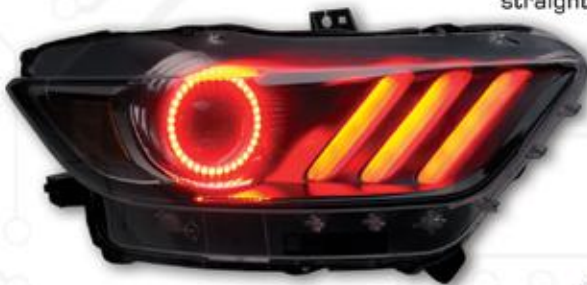
RGB 5050 Concept SMD strips installed as Daytime Running Lights behind the OEM diffusers.
