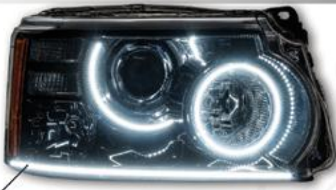
White Concept SMD strips installed as Daytime Running Lights.
