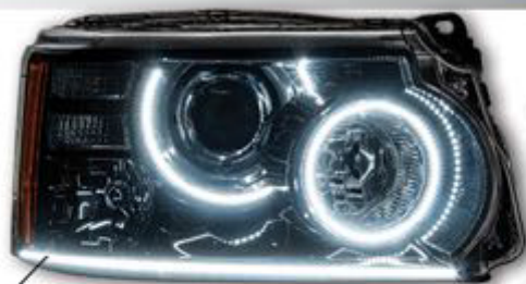
White Concept SMD strips installed as Daytime Running Lights.
